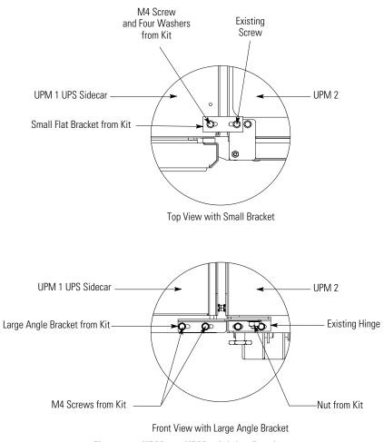
Figure 2-3. UPM 1 to UPM 2 Joining Brackets
